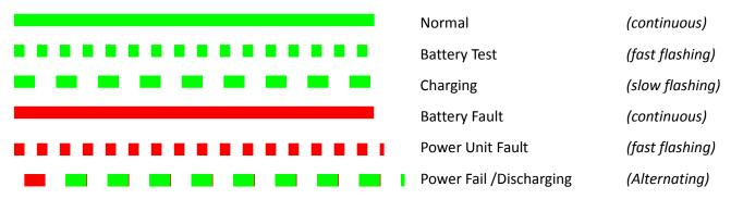
LED indicator is constantly Green - Operating correctly and the battery is fully charged.
