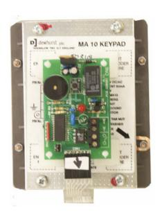
To program a number in to the KCA2. Press the program and \*button simultaneously a long bleep will sound the unit is now in program mode. Enter a four digit number for example (1234) followed by the \*key four short bleeps will sound. The unit has now got a security code number of 1234. Enter 1234 the LED will come alight on the back of the unit for two seconds which indicates the relay is energised for that period of time.
