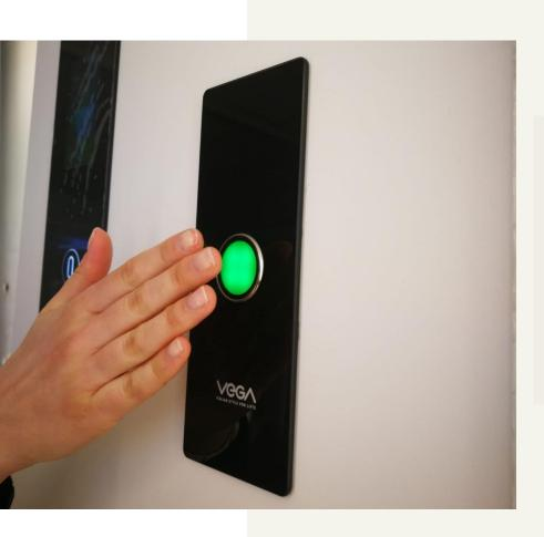
The new touch less push button by Vega that allows you to call the car only by approaching your hand thanks to a proximity sensor.
